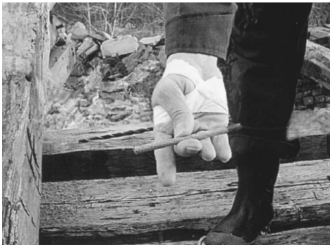
Figure 3 Bill Callahan displaying a sample from one of the D.P. and Jannetje (Deforest) Winne house first floor beams. Photograph Dec. 2003.
